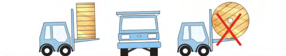
Lift drums on fork trucks correctly.
